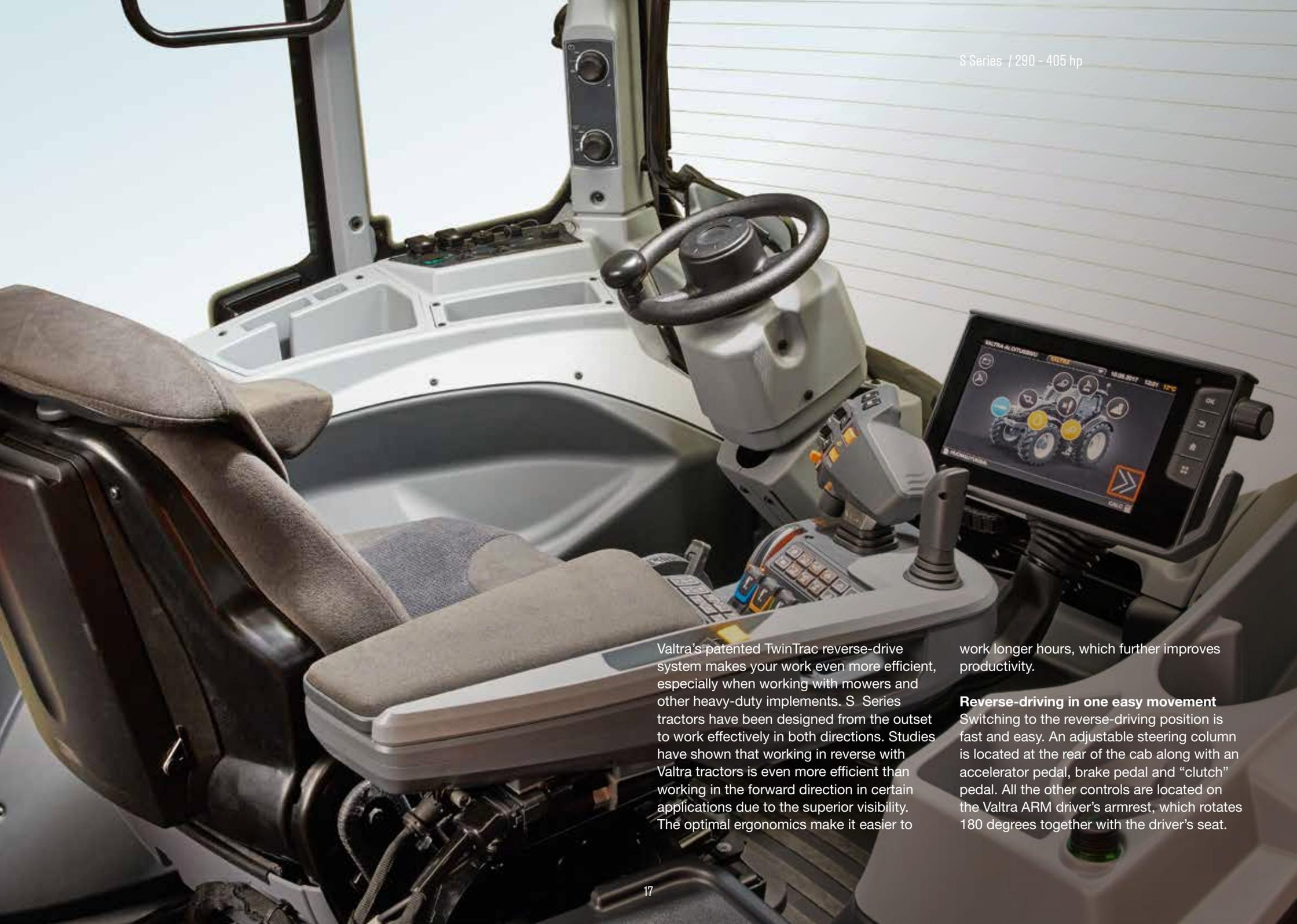
Valtra's patented TwinTrac reverse-drive system makes your work even more efficient, especially when working with mowers and other heavy-duty implements. S Series tractors have been designed from the outset to work effectively in both directions. Studies have shown that working in reverse with Valtra tractors is even more efficient than working in the forward direction in certain applications due to the superior visibility. The optimal ergonomics make it easier to
